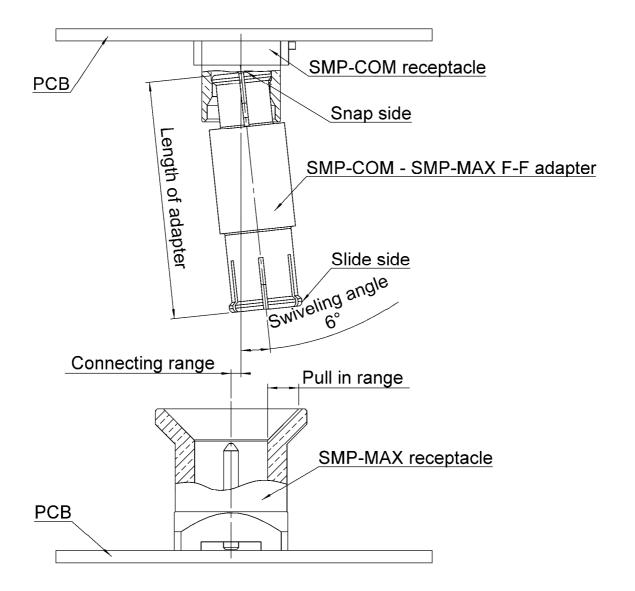
The connecting range represents the maximum misalignment during connection.
