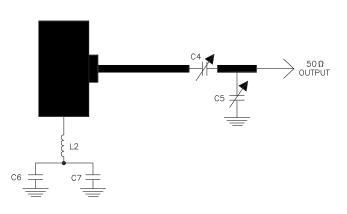
Material 1/32" Teflon Fiberglass C1,C3,C5 = .3-3.5 Johanson C2,C4 = .6-6 Johanson C6 = 82pf A.T.C.  $C7 = 200\mu f Electrolytic$  L1 = #18 AWG 0.6" LONG L2 = #18 AWG 1.0" LONG
