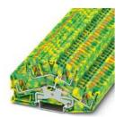
Protective conductor double-level terminal block, number of connections: 4, connection method: Push-in connection, 1st and 2nd level, cross section: 0.2 mm<sup>2</sup> - 6 mm<sup>2</sup>, mounting type: NS 35/7,5, NS 35/15, color: green-yellow
