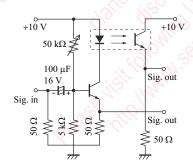
Measurement circuit of frequency characteristics
