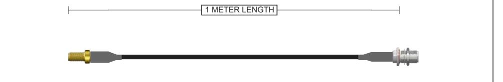
Connector A 132116 SMA Jack Straight Brass Gold + Heatshrink 50 Ohm RG-58 Continuity/Hi-Pot Connector B 082-5378 N-Type Jack Straight Bulkhead - Rear Mount Brass Nickel + Heatshrink
