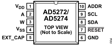
Figure 4. MSOP Pin Configuration
