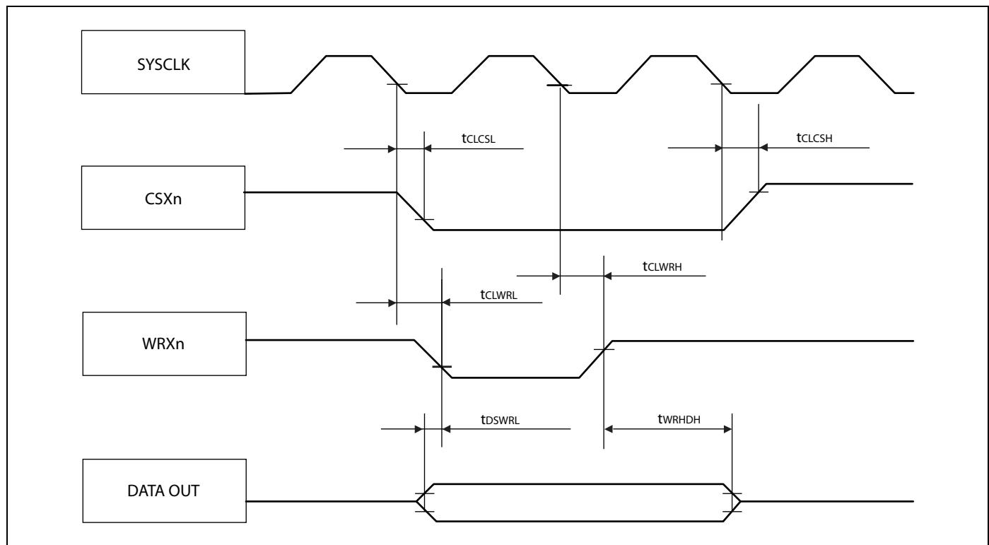
**Asynchronous write access - byte control type**
