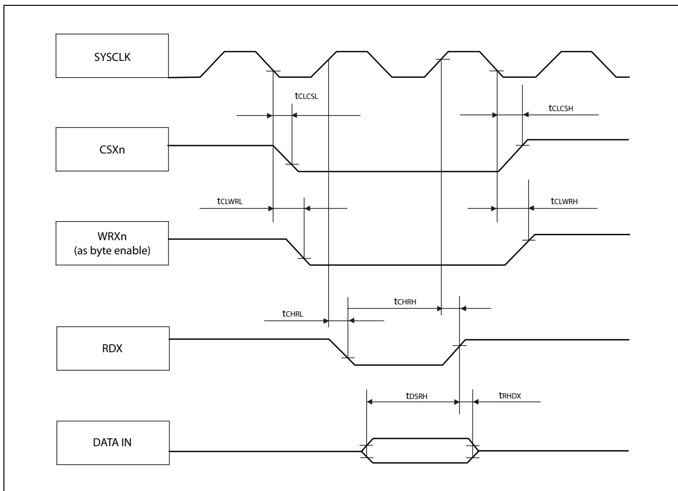
**Synchronous write access - byte control type**
