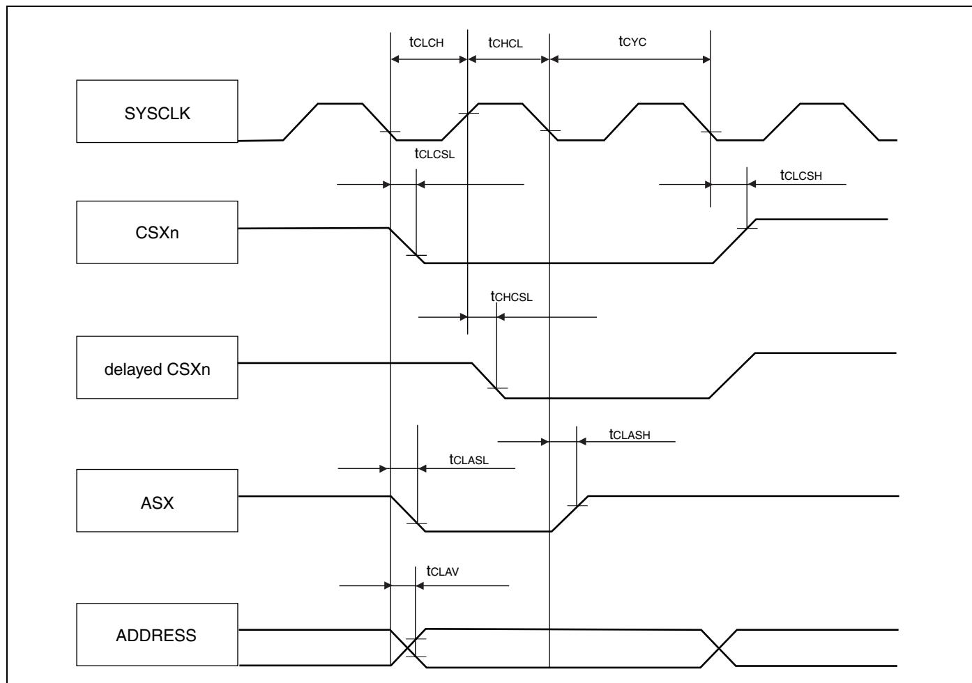
**Synchronous/Asynchronous read access**
