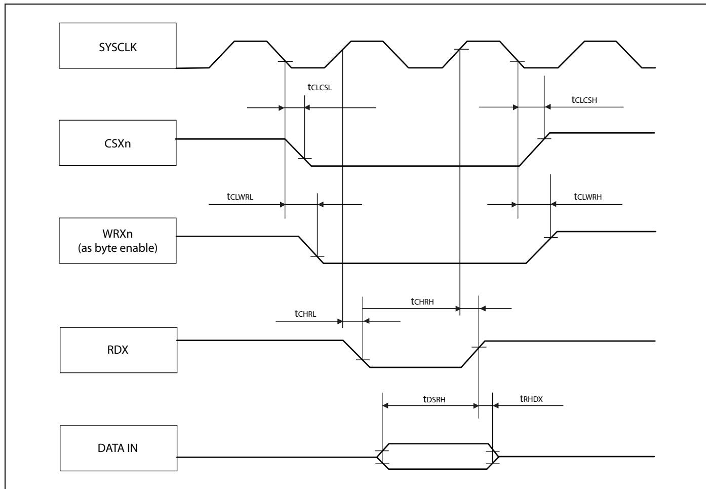
**Synchronous write access - byte control type**
