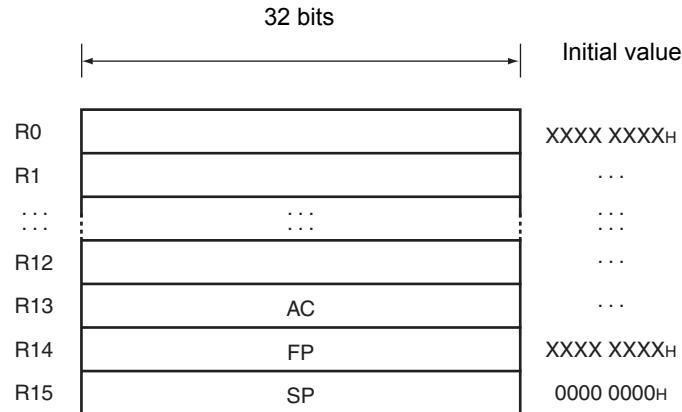
Registers R0 to R15 are general-purpose registers. These registers can be used as accumulators for computation operations and as pointers for memory access.
