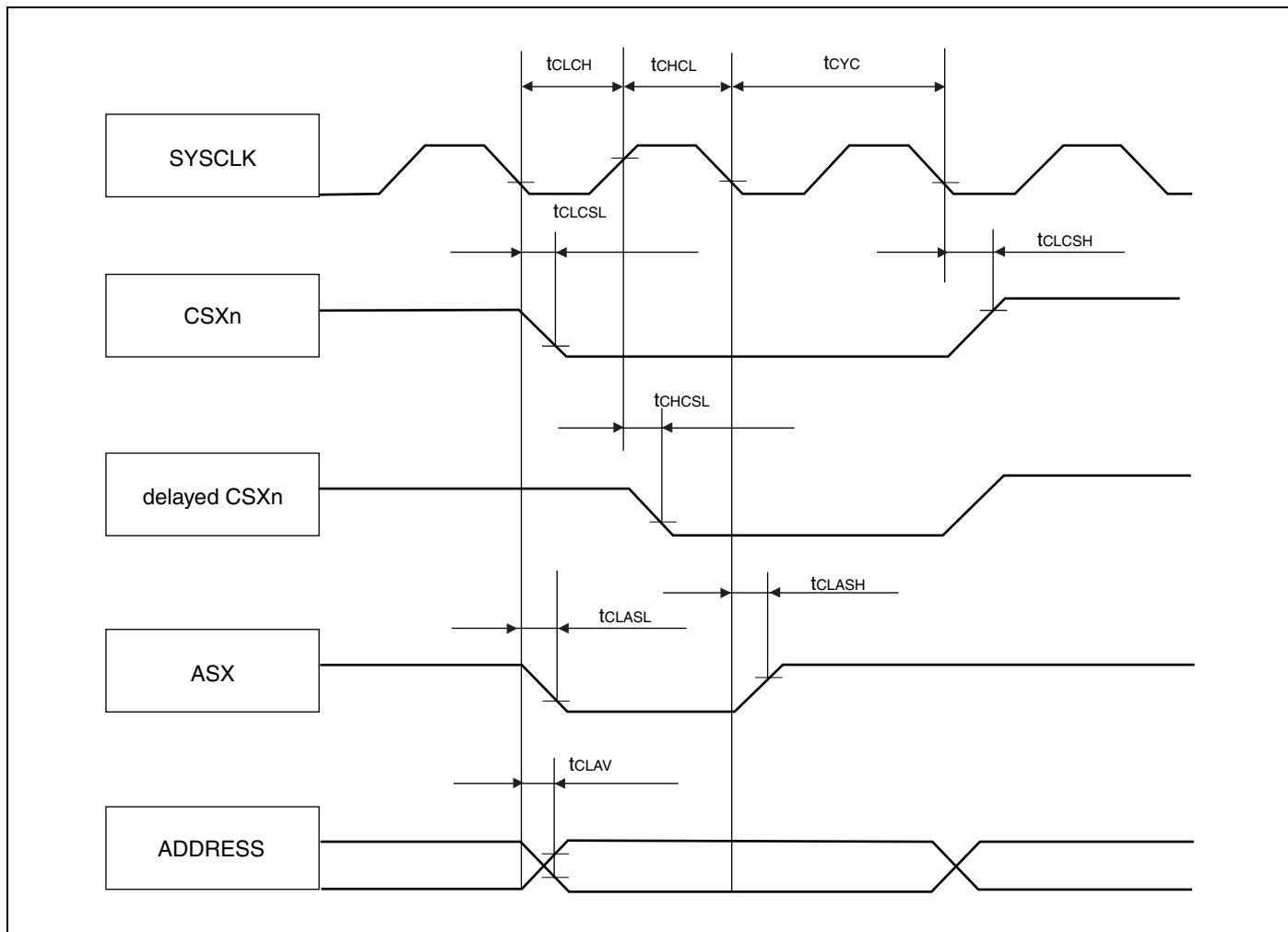
**Synchronous/Asynchronous read access**
