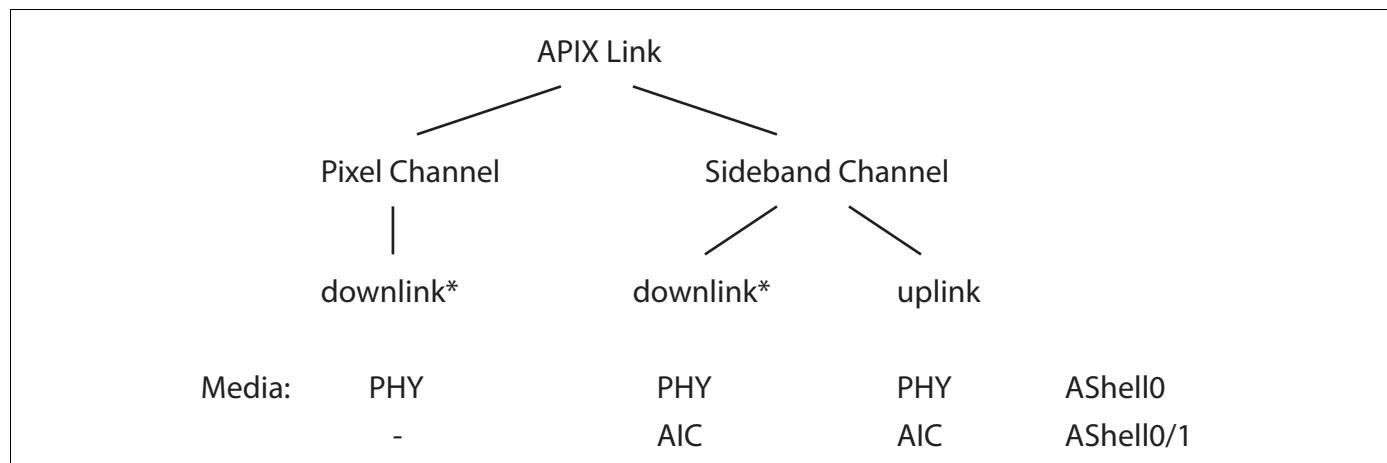
\*Remark: CY91460S series provides either downlink over Pixelchannel or over Sidebandchannel
