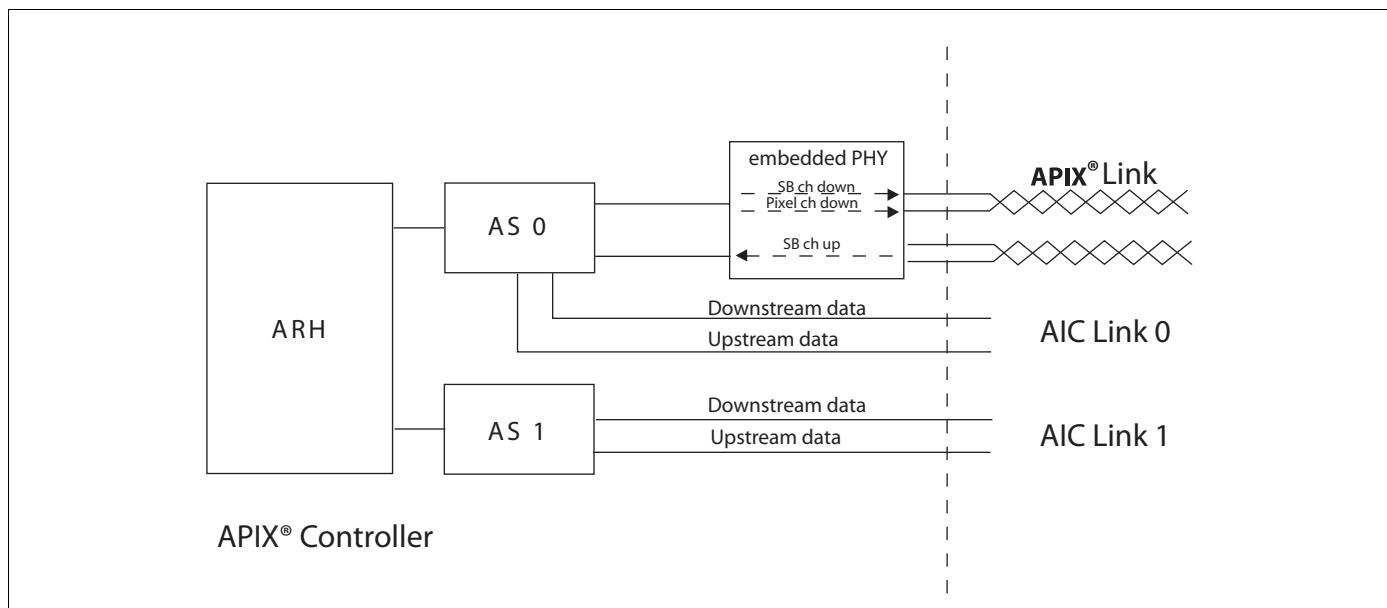
\*Remark: Link 1 can be used only if Link 0 is activated (CHCTRL: TXCFG = 0)
