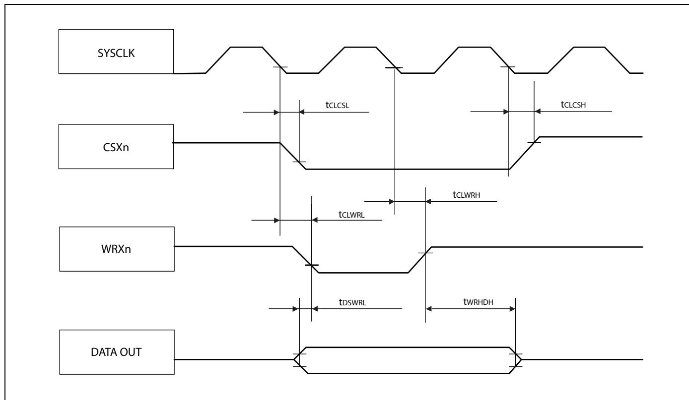
**Asynchronous write access - byte control type**
