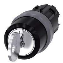
RONIS key-operated switch, 22 mm, round, plastic with metal front ring, lock number SB30, with 2 keys, 3 switch positions I-O-II, latching, actuating angle 2x45°, 10:30h/12h/13:30h, key removal O+I, possible special locks: SB31, 421, 455, with laser labeling, upper case
