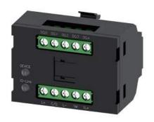
Electronics module IO-Link for ID key-operated switch, freely-programmable electronic switches, controller and RFID authentication of the switching function, black, operating voltage 24 V DC, screw terminal, for front plate mounting, for industrial application in control cabinets and machines
