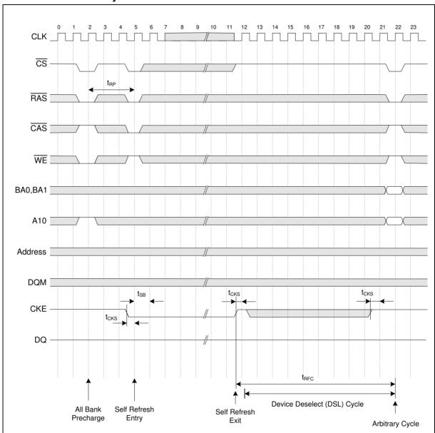
Note: The device exit the Self Refresh mode asynchronously at the rising edge of the CKE signal.
