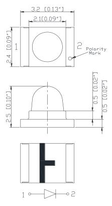
Units: mm / tolerance = +/-0.15mm
