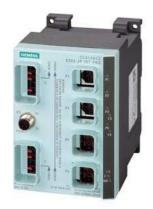
SCALANCE X202-2PIRT PRO, Managed IE IRT switch, Degree of protection IP65/67, 2x 10/100 Mbit/s Push Pull RJ45 ports, 2x 100 Mbit/s Push-pull SCRJ port; Error signaling contact with set pushbutton, Redundant power supply, PROFINET IO device; network management, Redundancy Manager integrated, incl. electron. manual on CD-ROM, C-plug optional.
