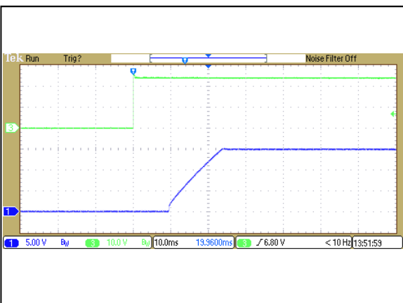
Figure 23: ATA02C18-L Output Voltage Startup Characteristic by Vin Vin = 24Vdc Load: Io = 0.535A Ch1: Vo Ch3: Vin
