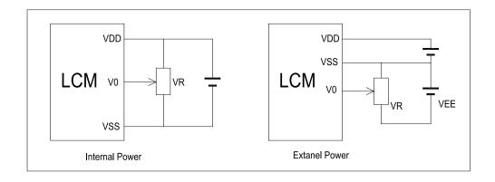
$V_{DD^{\sim}}V_0\text{: LCD Driving voltage}$
