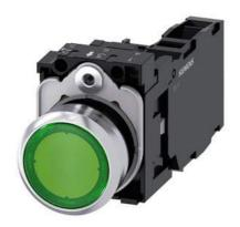
Illuminated pushbutton, 22 mm, round, metal, shiny, green, pushbutton, flat, momentary contact type, with holder, 1 NO+1 NC, LED module with integrated LED 24 V AC/DC, screw terminal
