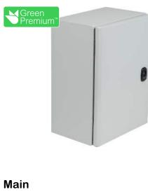
Wall mounted steel enclosure, Spacial S3DC, plain door, without plain chasis, 400x400x200mm, IP66, IK10
