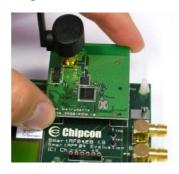
The CC2430-CC2590EM can be plugged into the SmartRF04EB. Please refer to the CC2430DK User Guide for more information about SmartRF04EB.
