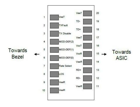
Pin-out of connector Block on Host board
