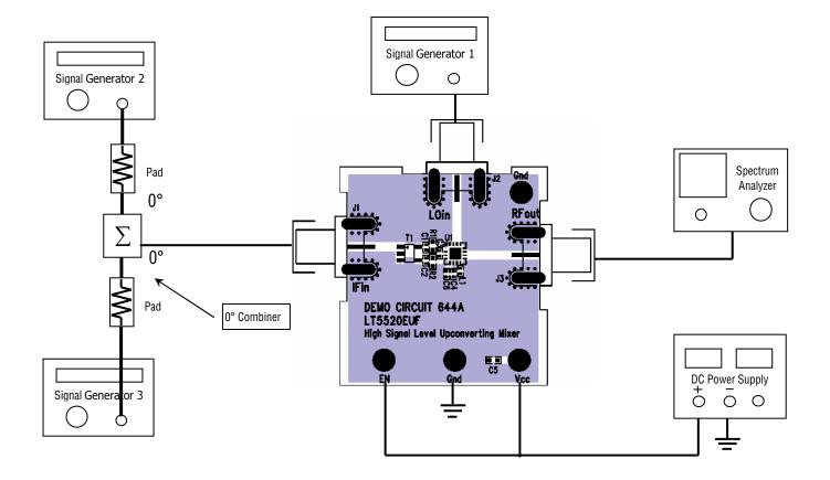
Figure 1. Proper Measurement Equipment Setup
