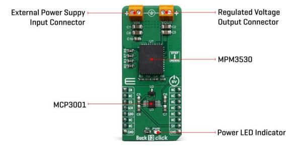
The output voltage is determined by the feedback voltage on the FB pin. Therefore, Buck 13 click is equipped with a fixed voltage divider calculated to ensure stable, the most frequently used, 3.3V output. The MPM3530 operates at very high switching frequency of 520 kHz, which allows a good compromise between the efficiency and the size of the device with no external coil needed and minimal number of other external components.
