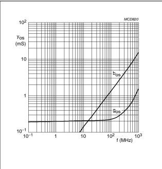
$V_{DS} = 8 \text{ V}; V_{GS} = 0; T_{amb} = 25 \,^{\circ}\text{C}.$
