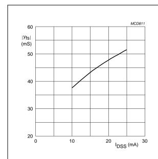
$V_{DS} = 8 \text{ V}; T_j = 25 \text{ }^{\circ}\text{C}.$
