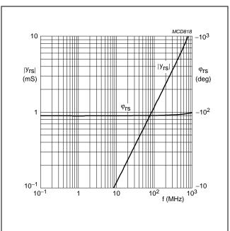
$V_{DS} = 5 \text{ V}; V_{G2} = 4 \text{ V}.$  $I_D = 15 \text{ mA}; T_{amb} = 25 ^{\circ}\text{C}.$
