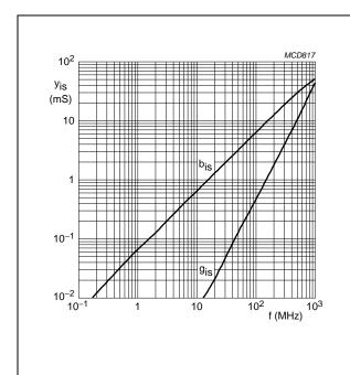
$V_{DS}$  = 8 V;  $V_{GS}$  = 0;  $T_{amb}$  = 25  $^{\circ}C.$
