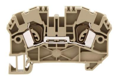
Feed-through terminal, Tension-spring connection, Mounting type: Mounting rail TS 35/7.5, Rated cross-section: 4 mm², Width: 6.1 mm, Colour: Beige
