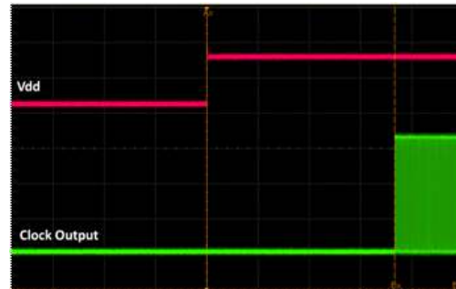
Figure 14. Startup Waveform vs. Vdd
