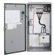
Enclosed soft starter, Controller 3RW44456BC34, Std. duty rating 200HP @460V, Std. duty current rating 280A Control voltage 115Vac Encl NEMA type 4X 304 S-steel Water/dust tight noncorrosive
