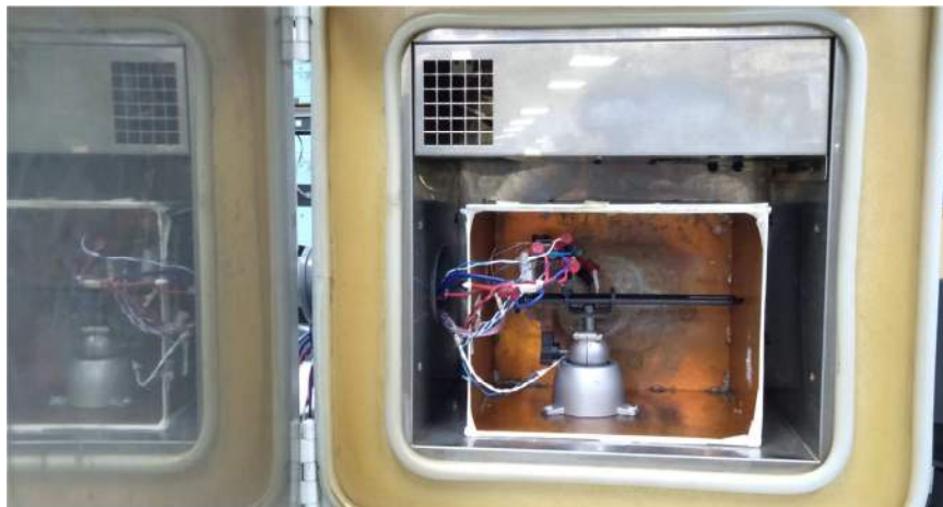
Figure 127 – Thermal Performance Set-up Using Thermal Chamber.
