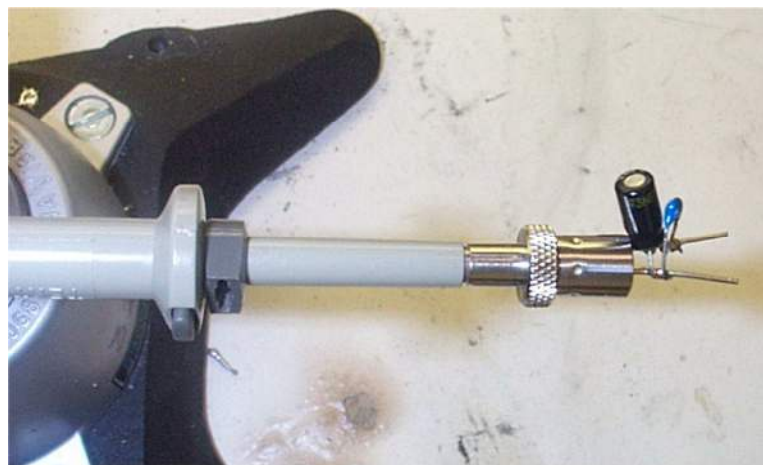
Figure 103 – Oscilloscope Probe with Probe Master ( www.probemaster.com ) 4987A BNC Adapter. (Modified with wires for ripple measurement, and two parallel decoupling capacitors added.)
