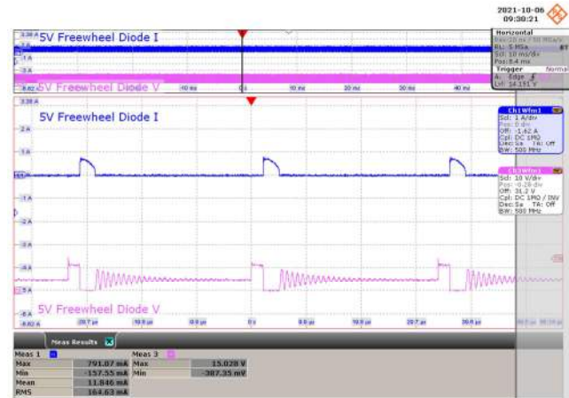
Figure 95 – 115 VAC 60 Hz. CH1: I_{5V\_Diode} , 1 A / div., 10 ms / div. CH3: V_{5V\_Diode} , 10 V / div., 10 ms / div. Zoom: 10 \mu s / div. PIV = 15.028 V, I_{D(MEAN)} = 0.011 A.
