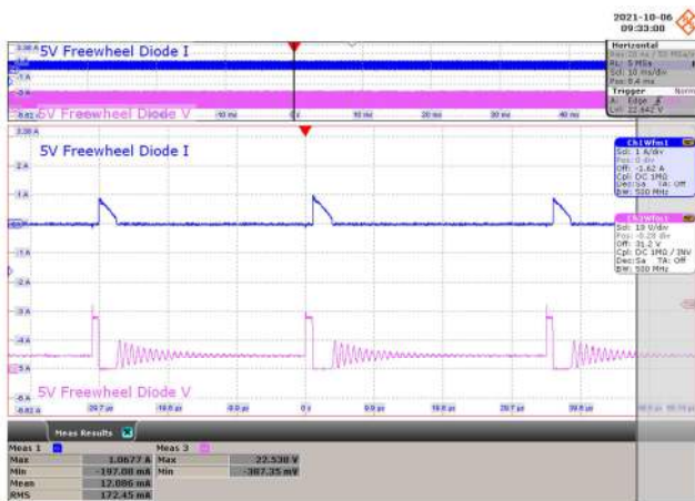
Figure 96 – 230 VAC 50 Hz. CH1: I_{5V\_Diode} , 1 A / div., 10 ms / div. CH3: V_{5V\_Diode} , 10 V / div., 10 ms / div. Zoom: 10 \mu s / div. PIV = 22.538 V, I_{D(MEAN)} = 0.012 A.
