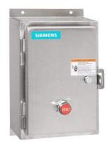
Non-reversing motor starter, Size 1, Three phase full voltage, Solid-state overload relay, OLR amp range 5.5-22A, 208VAC 60Hz coil, Non-combination type, Encl. type 4X 304 S. Steel, Water/dust tight noncorrosive, Standard width enclosure
