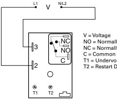
V = Voltage NO = Normally Open NC = Normally Closed C = Common T1 = Undervoltage Trip Point T2 = Restart Delay
