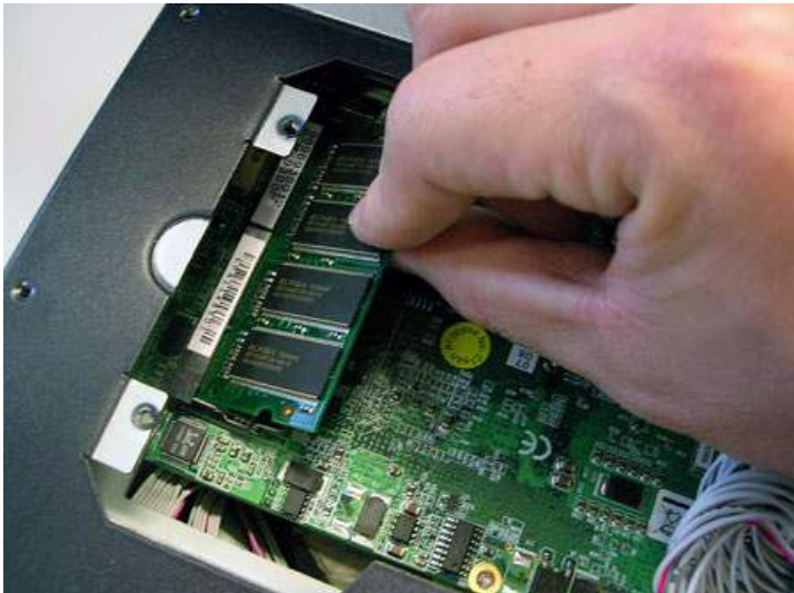
Figure 4.4: Plug the SDRAM into the RAM socket
