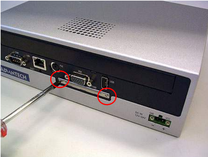
Figure 4.5: Unscrew CF carrier from front plate
