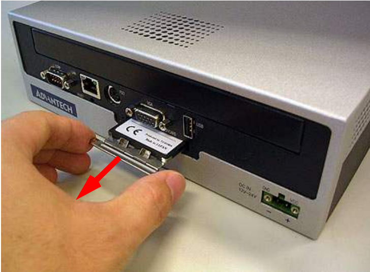
Figure 4.6: Unscrew CF carrier from the front plate
