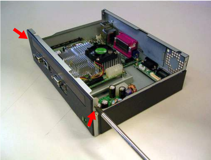
Figure 5.10: Remove the expansion IO plate on the front panel
