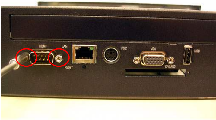
Figure 5.7: Unscrew the Hex-bolts of the front cover (ex: EBPC-3500-80SE)
