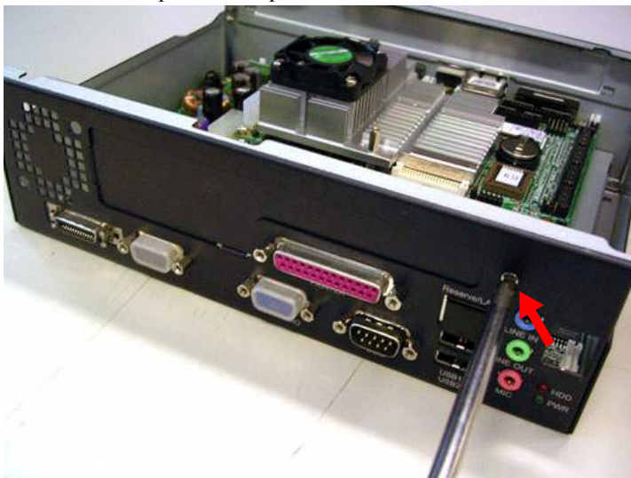
Figure 5.11: Remove the expansion IO plate on the rear side
