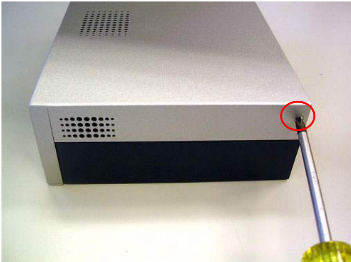
Figure 5.1: Unscrew top cover (right screw)
