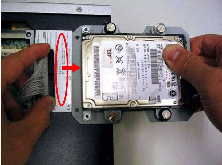
Figure 4.9: Connect the IDE cable to the HDD connector
