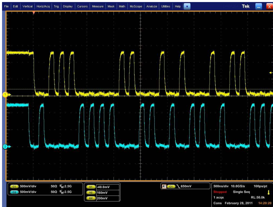
Figure 8. EMI4183 MIPI D-PHY LP Mode Measured Results
