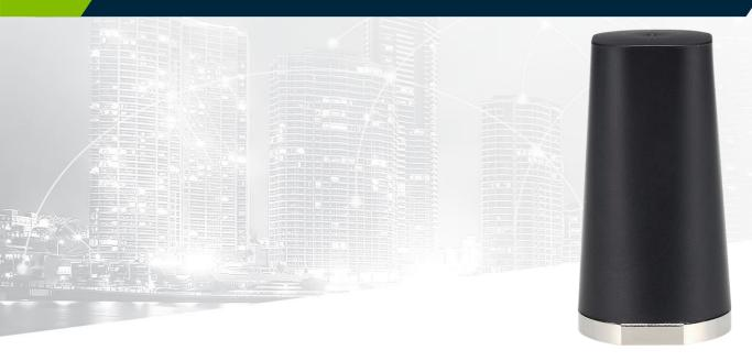
The Shockwave TLS.20.1F11 is a mechanically robust, waterproof, external antenna operating at the 450-470MHz with 1 meter low loss TGC-200 cable and SMA(M) connector. It has been designed to be used on a ground plane.
