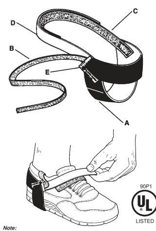
Two heel straps are recommended for reliable grounding and ESD protection, providing ground when one foot is off the floor.
