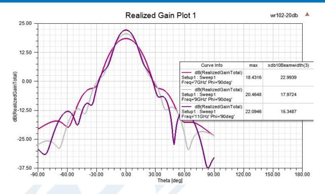
WR-102 Standard Gain Horn with 20 dBi gain, N Female connector from Pasternack Enterprises has same day shipment for domestic and International orders. Our RF, microwave and millimeter wave products maintain a 99.4% availability and are part of the broadest selection in the industry.
