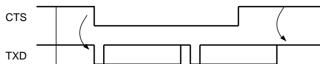
Figure 31-21. Transmitter Behavior when Operating with Hardware Handshaking
