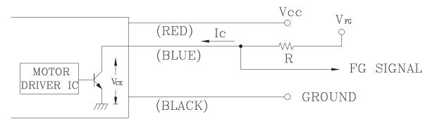
CAUTION: THE FG SINGAL LEAD WIRE MUST BE KEPT AWAY FROM "+" LEAD WIRE & "-" LEAD WIRE.
