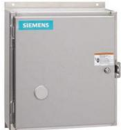
Mechanically held lighting contactor, Contactor amp rating 30Amp 0NC  $\_$  3NO poles, 24VAC 60HZ coil, Non-combination type, Encl NEMA type 4X 304 S-steel Water/dust tight noncorrosive
