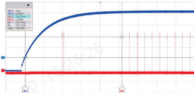
Figure 5-5 Sample5 Start-Up Time Test Curve
