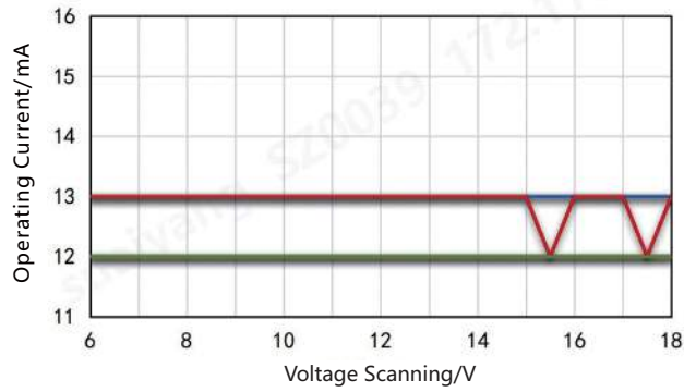
Figure 5-9 -40°C Current Consumption Test Curve
