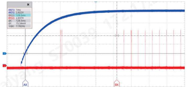
Figure 5-4 Sample4 Start-Up Time Test Curve
