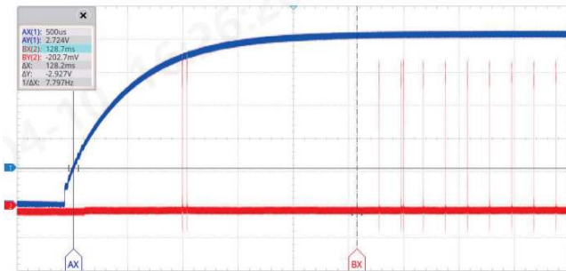
Figure 5-7 Sample7 Start-Up Time Test Curve
