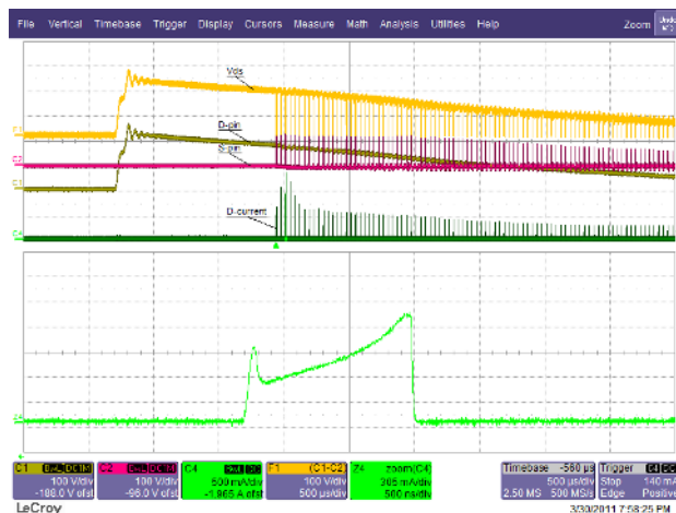
Figure 34 – 150 °C Start-up; 135 VAC / 63 Hz; 85° Phase Angle, 35 V LED String.
