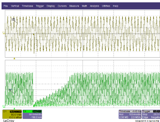
Figure 44 – 115 VAC / 50 Hz, 0.25 Cycle-Skip. Load: 35 V LED String. Ch1: V_{IN} , 50 V / div. Ch3: I_{IN} , 50 mA / div., 100 ms / div.
