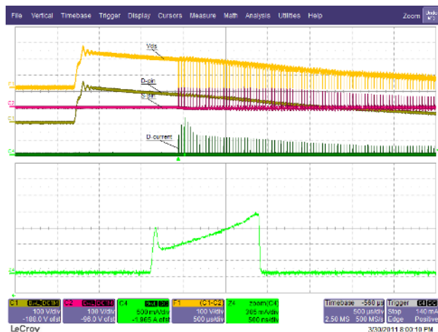
Figure 33 – 125 °C Start-up; 135 VAC / 63 Hz; 85° Phase Angle, 35 V LED String.
