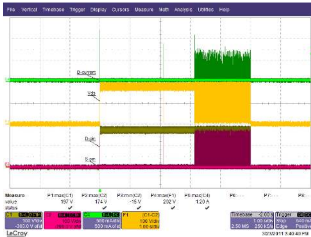
Figure 37 – 135 VAC / 63 Hz, Output Shorted. Ch1: V_{DRAIN} , 100 V / div. Ch2: V_{SOURCE} , 100 V / div. Ch4: I_{DRAIN} , 0.5 A / div. F1: V_{D-S} , 100 V / div., 1 s / div.
