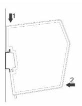
Make sure the DIN-rail fastening mechanism on the back of the module is in a fixed and closed position, i. e. pushed all the way up.
