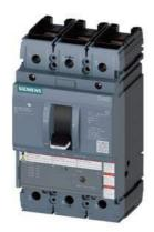
circuit breaker 3VA5 UL frame 250 3-pole, starter protection TM120M, AM, In=200A without overload protection short-circuit protection li=3...6 x In nut keeper kit on both sides
