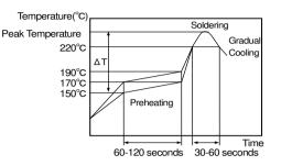
[Standard Conditions for Reflow Soldering]
