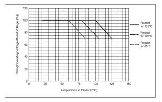
These Part Numbers are designed for use in the circuits where continuous applied voltage to the capacitor is derated than rated voltage, and guarantee Durability Test with 100% × rated voltage as testing voltage at the maximum operating temperature. The voltage and temperature derating conditions on the left are recommended for use to ensure the same reliability level as normal specification.
