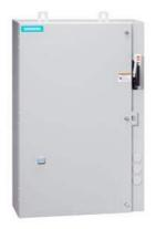
Non-reversing motor starter, Size 2 1/2, Three phase full voltage, Solid-state overload relay, OLRelay amp range 25-100A, 208VAC 60HZ coil, Combination type, 100A non-fusible disconnect, Enclosure NEMA type 4/12, Water/dust tight for outdoors, Standard width enclosure
