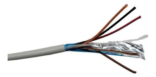
These 24AWG (American Wire Gauge) 4 bare copper conductor stranded-shielded cables can be used for a wide variety applications, including: security/alarm, sound and audio, background music and power-limited control circuits.
