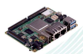
The i.MX8 Quad MAX/Quad Plus Pico ITX SBC integrates Dual Cortex A72 + Quad Cortex A53 Cores, Dual GPU systems,
