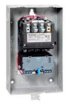
Non-reversing motor starter Size 1 Three phase full voltage Solid-state overload relay OLRelay amp range 0.25-1A 220-240/440-480VAC 60HZ coil Combination type Indoor general purpose use
