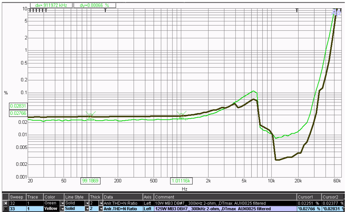
Figure 4 THD+N vs. Frequency at 10W and 125W
