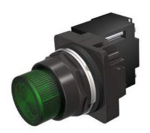
30mm BlackMax, Epoxy Coated Corrosion Resistant Complete Metal Unit Illuminated Indicator Light Transformer type, 240V AC LED Lamp, BA9s Plastic Lens, Green UL Listed, CSA Certified NEMA 1,3,3R,4,4X,12,13 & Automotive Standards
