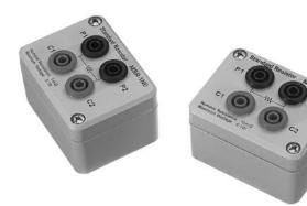
electromotive force, respectively. The MSR is a compact suitable standard resistor for daily calibration of milliohm meters, etc. Although the MSR series is a low cost, easy to use product, it offers both high stability and low temperature coefficient. The MSR is most suitable as a standard resistor to be used on the job site.
