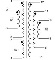
$N1,\,N2$  denotes windings connected in parallel. Terminals 1+2, 5+6, 7+8+9 and 10+11+12 must be tied as solder bridging is allowed.
