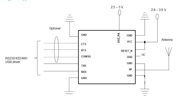
Note that the VCC\_PA pin supply the internal power amplifier only, while the rest of the internal block runs on VCC. They can be connected together or separated using individual supply. If VCC\_PA is connected together with VCC, the max output power is reduced to +24 dB for all modules except RC1701HP that support +27 dBm at VCC\_PA = 3.3 V. For all low power variant the VCC\_PA pin can be left open.
