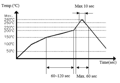
\* Reflow profile of lead-free solder
